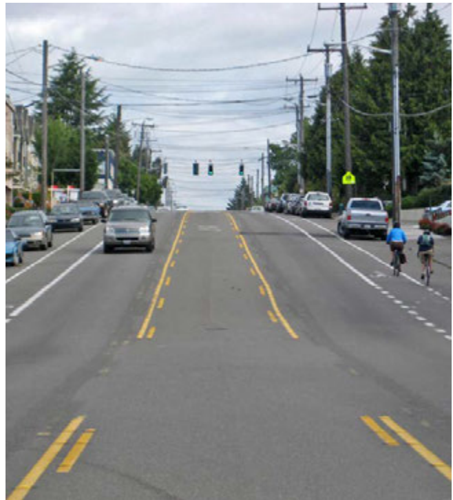
Figure 36: Two-Way Left-Turn Lanes
