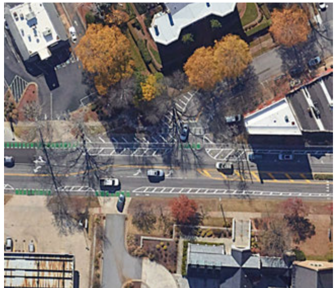
Figure 77: After: The skewed intersection was straightened with corners that have a smaller radius, thereby reducing the speed of turning vehicles, and reducing the crossing distance for pedestrians.
