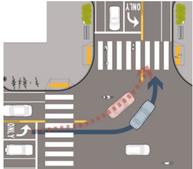
Figure 35: Hardened centerlines promote wider left turns by motor vehicles, thereby enhancing visibility for pedestrians crossing the street.
