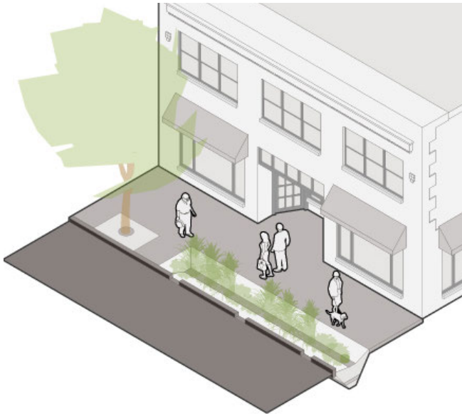
Figure 26: Green infrastructure encompasses various features like bioswales, which effectively capture and filter stormwater runoff.
