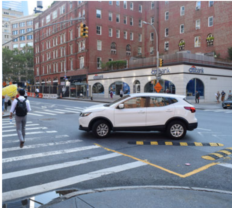
Figure 61: Turn wedges at intersections use low-cost materials like paint and rubber to slow turns and protect cyclists and pedestrians.
