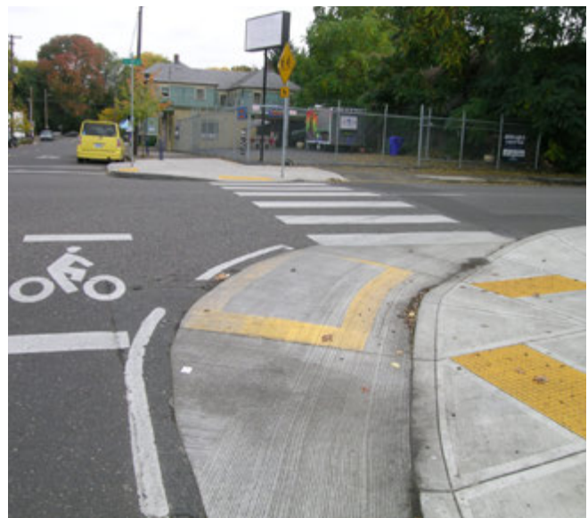
Figure 59: Mountable truck aprons facilitating turns for all vehicles to optimal corner radii ensuring comfortable driving speeds.
