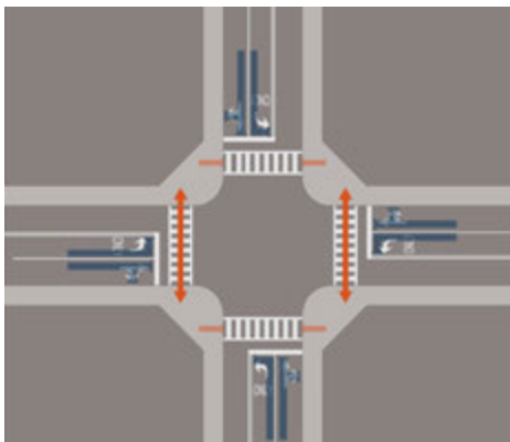
Figure 70: Leading Pedestrian Interval Phase 1
